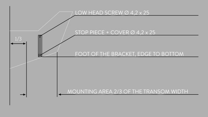
When mounting the transducer bracket, make sure that the transducer sensor is not straight on the line of the lifting strake. This causes a swirl, which then might give the sensor wrong information.
